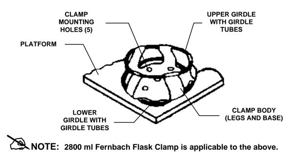
NBS flask clamps are used on a variety of shaker platforms. Flat head screws of different lengths and thread pitch are used to secure the clamp. The following tables identify the proper screw for your shaker application by reference to the head style.
