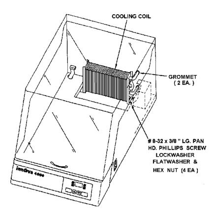
Figure 10b Cooling Coil Installation
