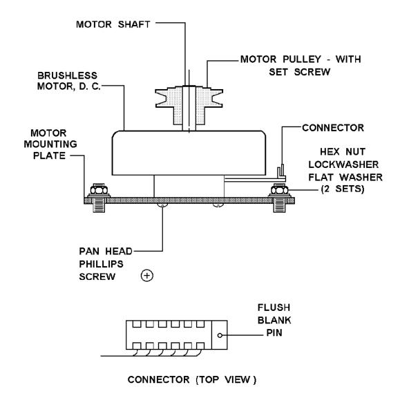
Figure 8 Motor Assembly Replacement
