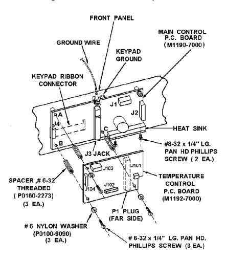
Figure 11 Control Board Replacement
